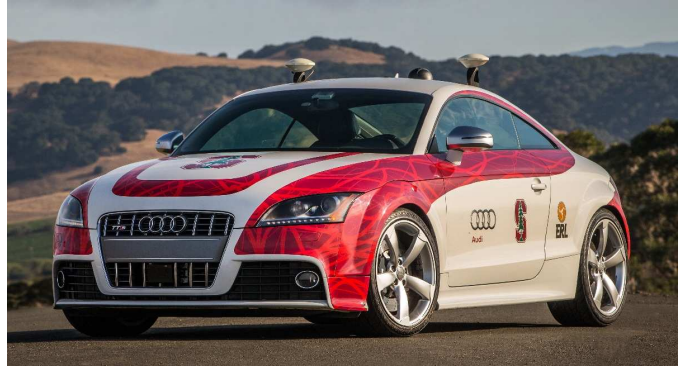
Fig. 3. Autonomous Audi TTS used for vehicle control research at the limits of friction
