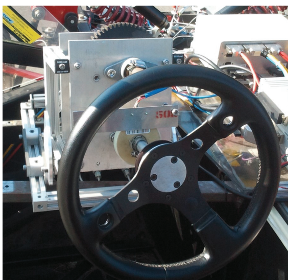
Figure A.1: FFB steering system mounted on X1
